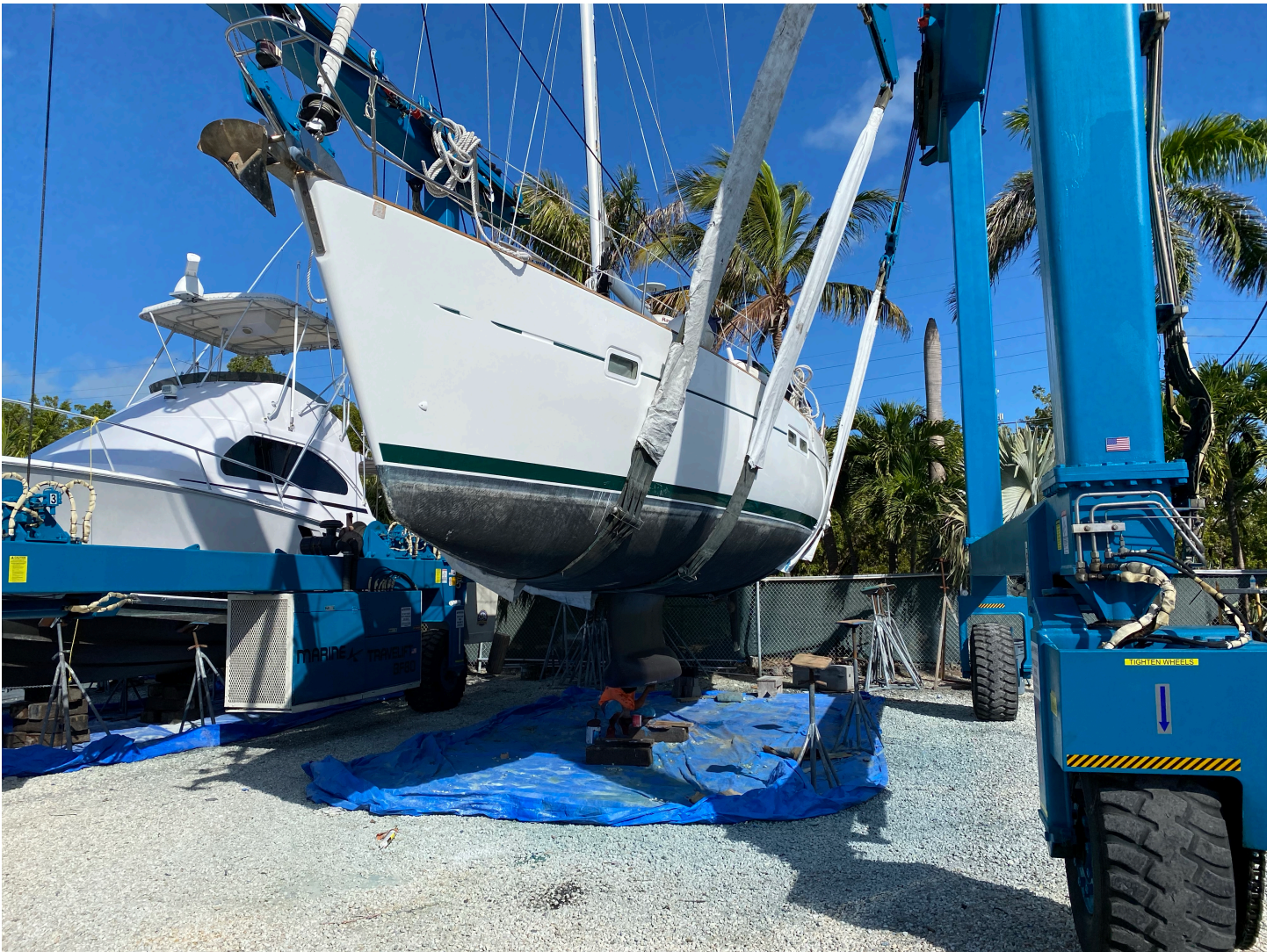
Fig 7: Note bow high in the slings
